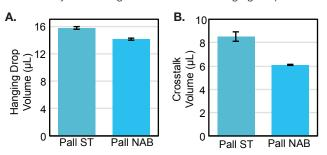
Hanging-drop (A) and crosstalk (B) volumes for the Pall NAB plate and Pall's previous generation plasmid DNA purification plate (Pall ST: PN 8132). For hanging-drop volume, the total hanging drop volume was determined for three plates, and the average volume/well calculated. For crosstalk volume, the data represents the average of 216 data points.
